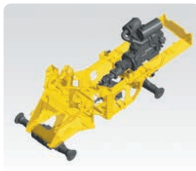
Robust torsion-resistant main frame
