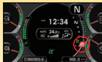
AdBlue® level gauge and refill guidance
