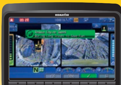
Eco-gauge, Eco guidance and fuel consumption gauge
