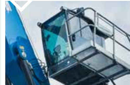
CATWALK WITH HANDRAIL*
